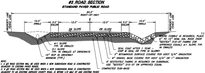
2. A 45 HOAD SECTION WILL BE USED WHEN A NEW SUBDIVISION ROAD IS CONSTRUCTED ADJACENT TO AN EXISTING UNPAVED COUNTY ROAD, IS WITHIN 1/2 MILE OF AND EXISTING PAVED ROAD, AND THE COUNTY HAS PLANS TO PAVE THE CONHECTING ROAD WITHIN THE NEXT 3 YEARS. 3. SUBDIVISION LOTS TO BE 1 ACRE OR LARGER.
